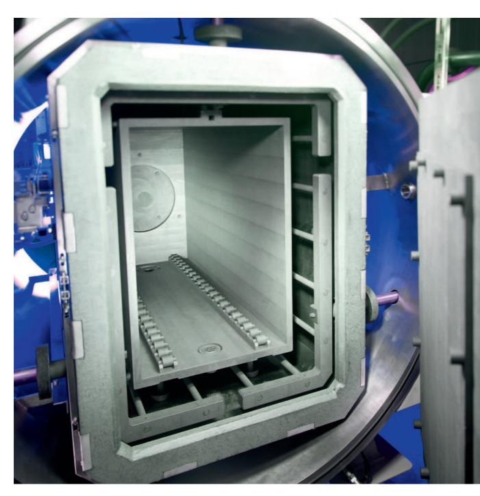
Vacuum - Heat Treatment and Sintering Furnaces COV
